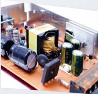
SW power supply
